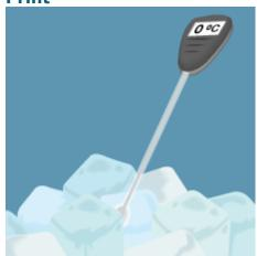
Temperature is a measure of how hot or cold things are. You need a **thermometer** to measure temperature.
